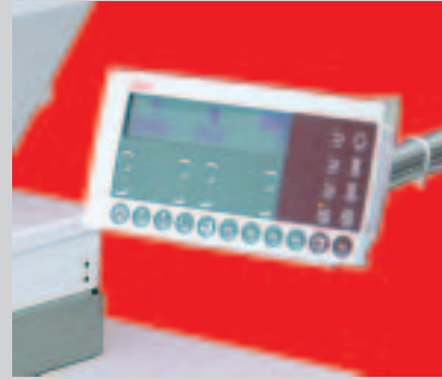
New S3 control panel with integrated data reader (SD-card) for importing sewing programs or machine software
